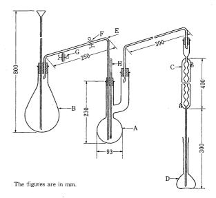
A: Distilling flask of about 300-mL capacity.
