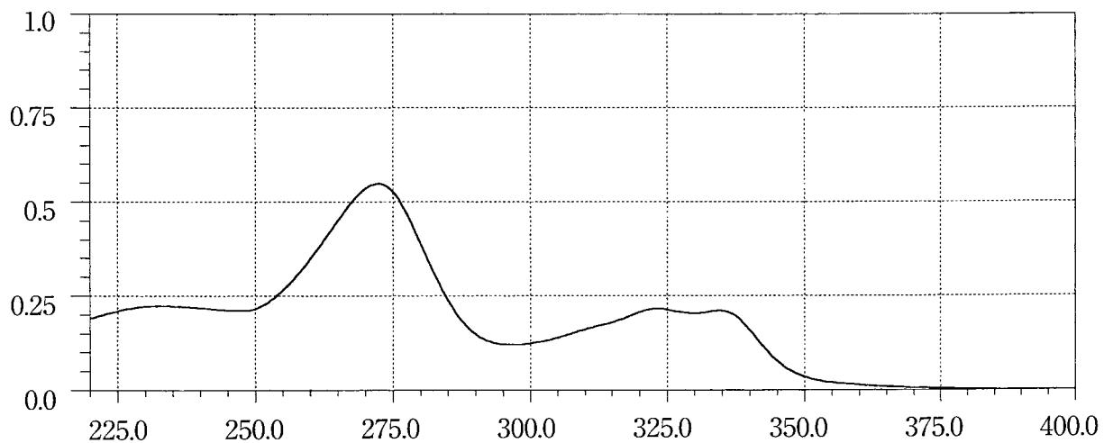
A solution prepared as follows: Dissolve 0.01 g of Norfloxacin in the aqueous solution of sodium hydroxide (1 in 250) to make 100 mL. To 5 mL of this solution add a solution of sodium hydroxide (1 in 250) to make 100 mL.
