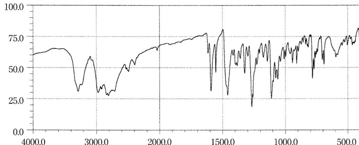
Preparation of sample: Potassium chloride disk method
