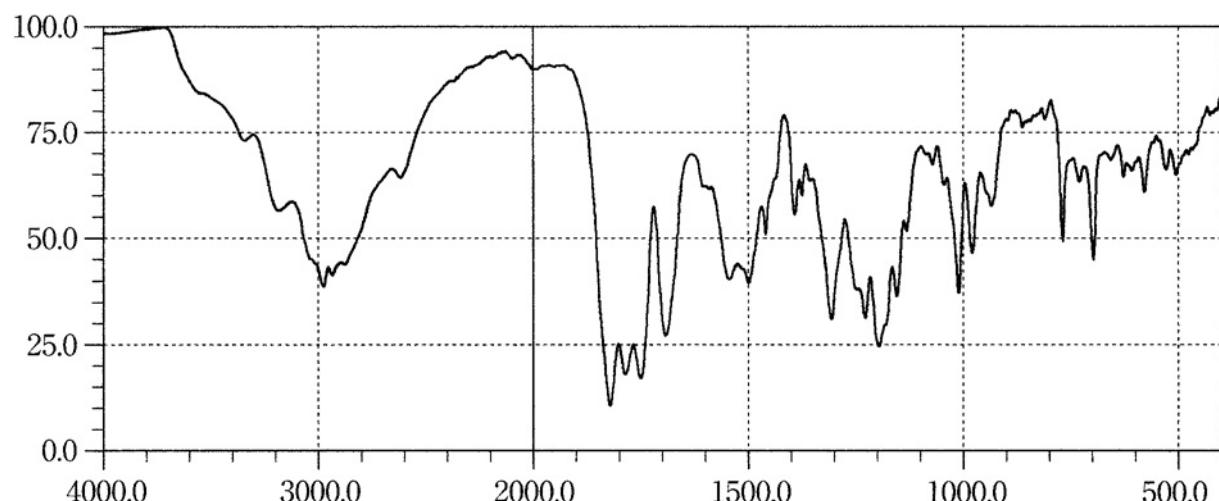
Preparation of sample: Potassium chloride disk method
