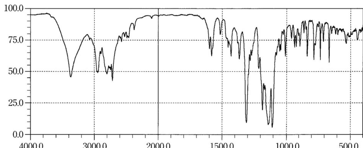
Preparation of sample: Potassium chloride disk method
