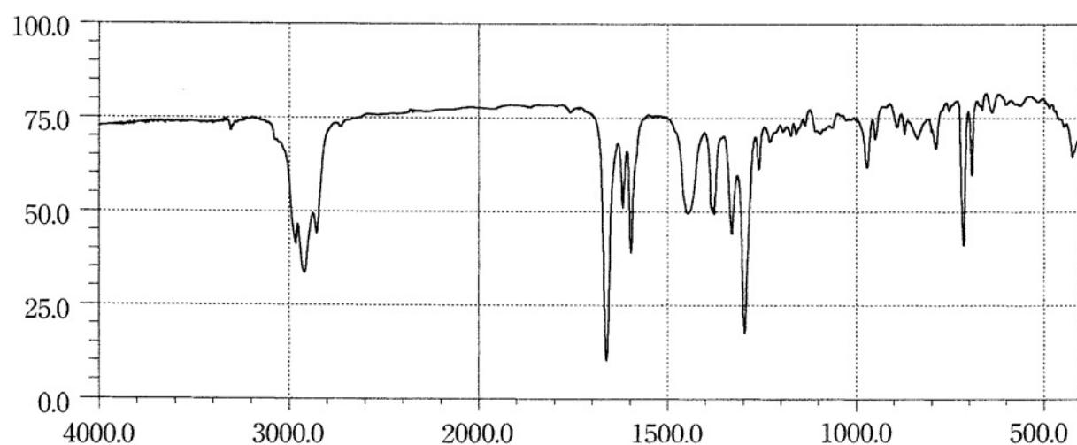
Preparation of sample: Liquid film method
