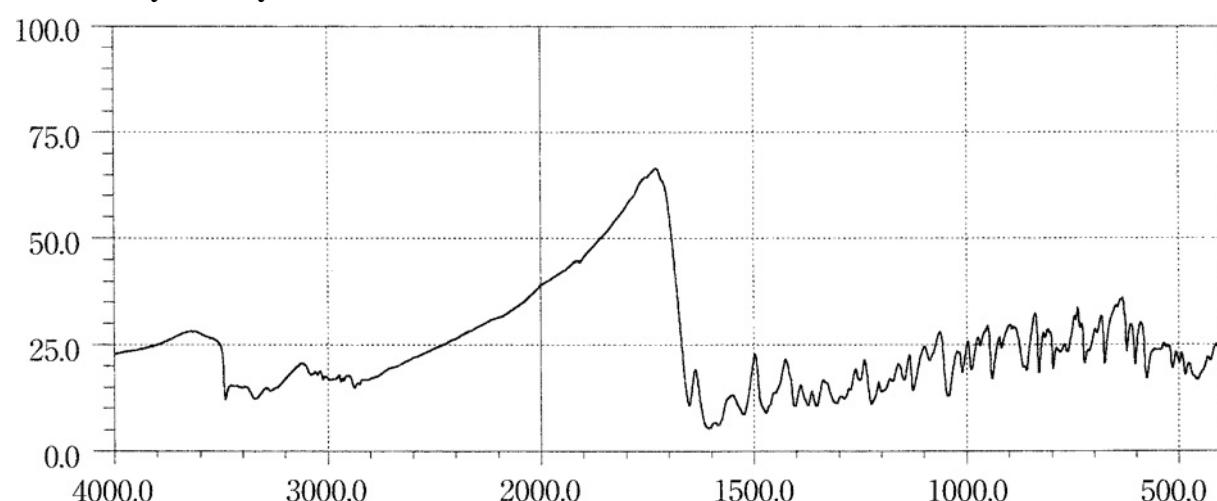
Preparation of sample: Potassium chloride disk method
