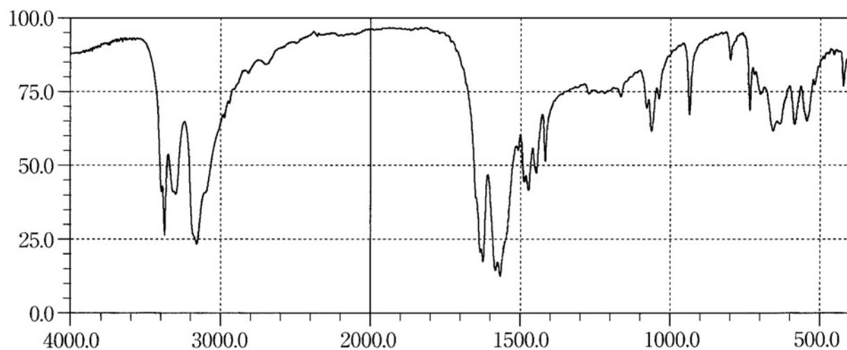
Preparation of sample: Potassium chloride disk method
