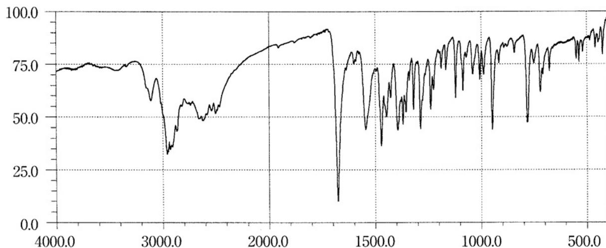
Preparation of sample: Potassium chloride disk method
