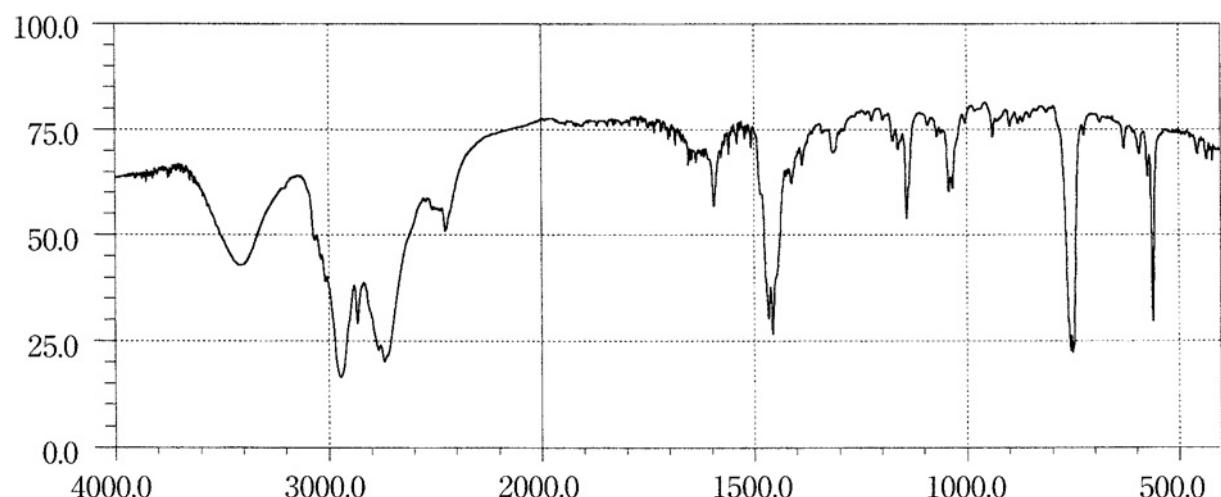
Preparation of sample: Potassium chloride disk method
